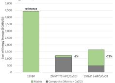
**Figure 3:** Reduced cost of thermal energy storage (\$/GJ) at the material-level through composite TCM development.
