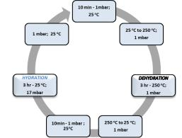
**Figure 2:** Procedure of **e**xperimental conditions for thermal properties characterization.
