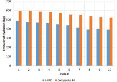
**Figure 4:** Preliminary cycling stability testing of J-HPC and corresponding composite #4.
