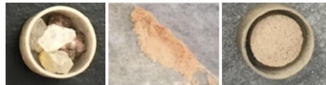
Figure 1: Shapes of natural zeolite samples tested in the form of a) granules b) powder and c) pellet.
